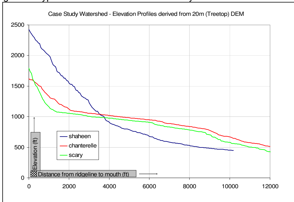
Figure 1. Hypsometric curves for the case study watersheds
